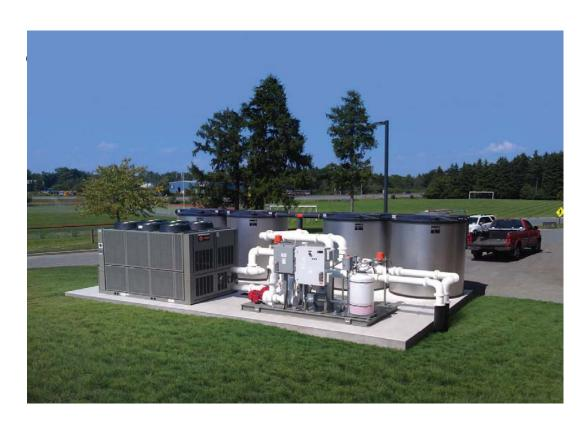
Skid mounted chiller plant - 200-ton peak cooling capacity with 90-ton, air-cooled, scroll chiller, pumps, controls and four ice thermal storage tanks
