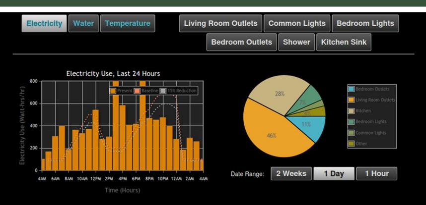
At the current rate: You will use 15% less electricity this hour than was typical for the same hour of day during the baseline period. Tip of the day: Reducing the amount of time spent in the shower by just 2 minutes can save 5 gallons of water!
