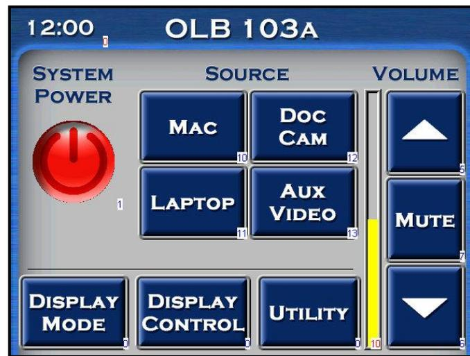
From the main page, you can power on the system, select the source to display, adjust the volume and navigate to the display mode, display control and utility pages.
